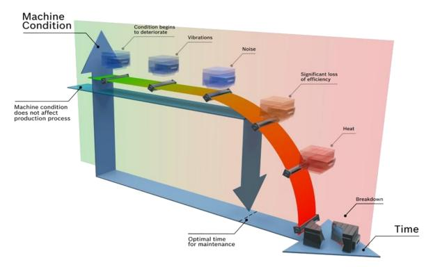
Figure 11: Prediction of machine condition and health index
