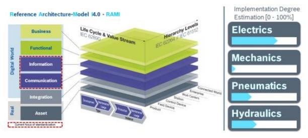
Figure 2: Reference Architecture Model I4.0 (RAMI)
