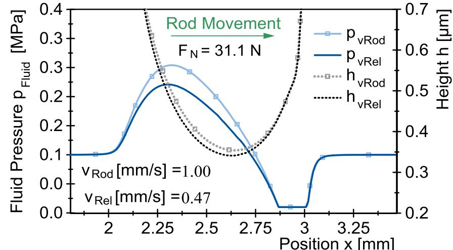
Slightly higher breakaway friction force due to lower fluid pressure
